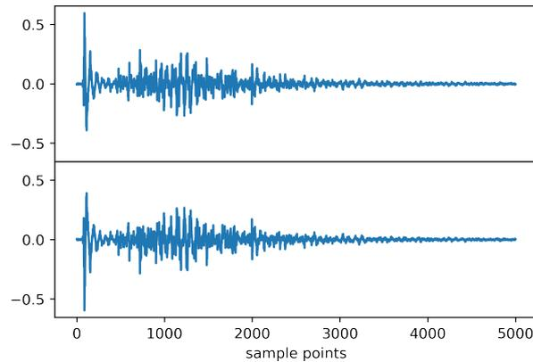
**Figure 5:** CPA on Software Implementation. The upper one is a random guess, and the lower one is the correct guess
