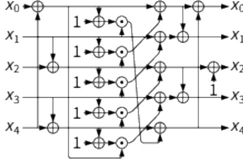
**Figure 4:** SBox of Ascon permutation
