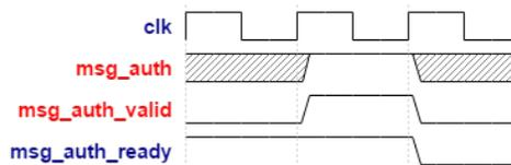
Figure 5.6: An example of a handshake used to perform message authentication
