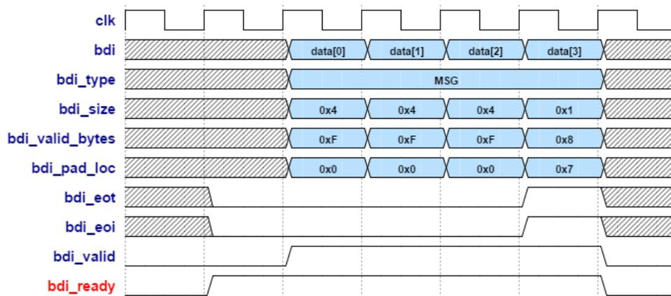
Figure 6.5: Handshake example of loading a message, for  $w=32$ , with data[3] containing the last 1 byte for encryption mode
