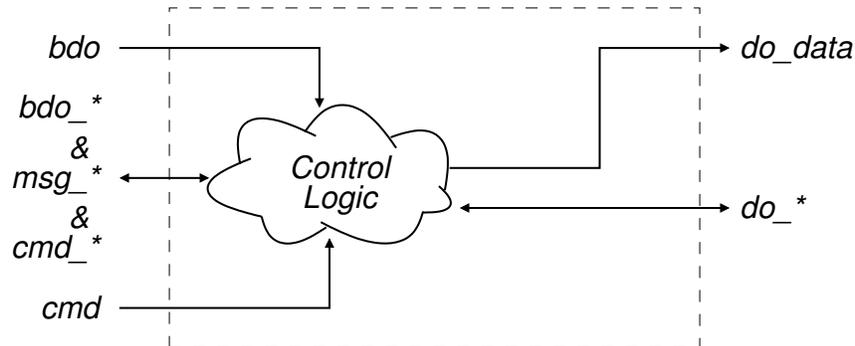
Figure 2.7: The *PostProcessor* Design.  $msg\_*$ ,  $cmd\_*$ ,  $bdo\_*$ , and  $do\_*$  stand for all the *PostProcessor* ports, shown in Figs. 2.5 with the names starting from the respective strings.
