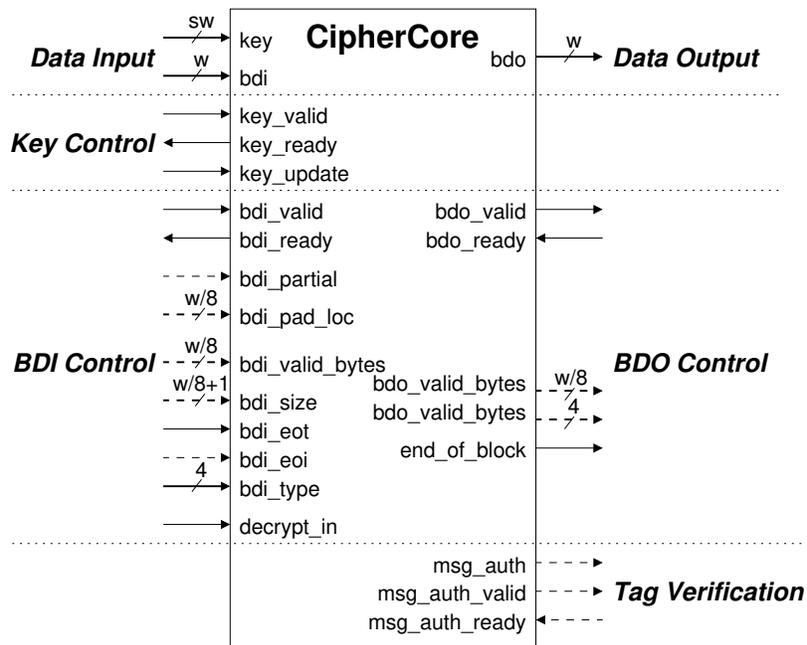
Figure 6.1: Interface of CipherCore for Lightweight Implementations.
