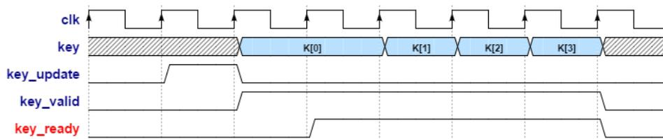
Figure 6.2: Handshake example of loading a key, for *sw*=32
