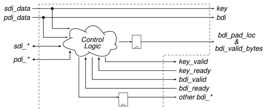
Figure 2.6: The *PreProcessor* Design. *pdi\_\** and *bdi\_\** stand for all the *PreProcessor* ports, shown in Figs. 2.5, with the names starting from the respective strings.
