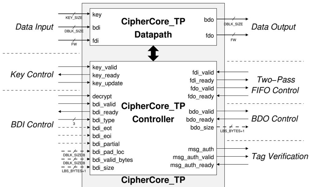
Figure 5.2: Interface of Two-Pass CipherCore
