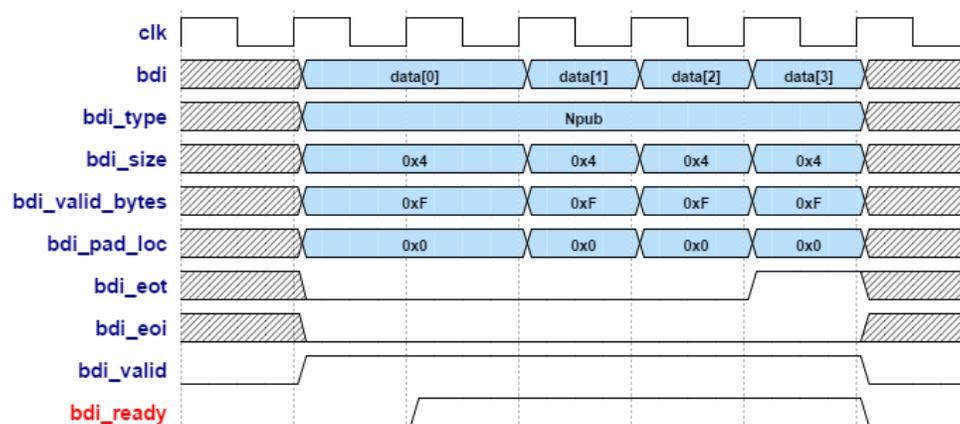
Figure 6.3: Handshake example of loading  $N_{pub}$ , for  $w=32$
