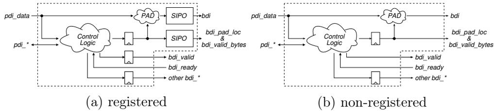
Figure 2.3: The PreProcessor Design. SIPO = Serial-In Parallel-Out unit.  $pdi\_*$  and  $bdi\_*$  stand for all PreProcessor ports, shown in Fig. 2.1, with the names starting from the respective strings.
