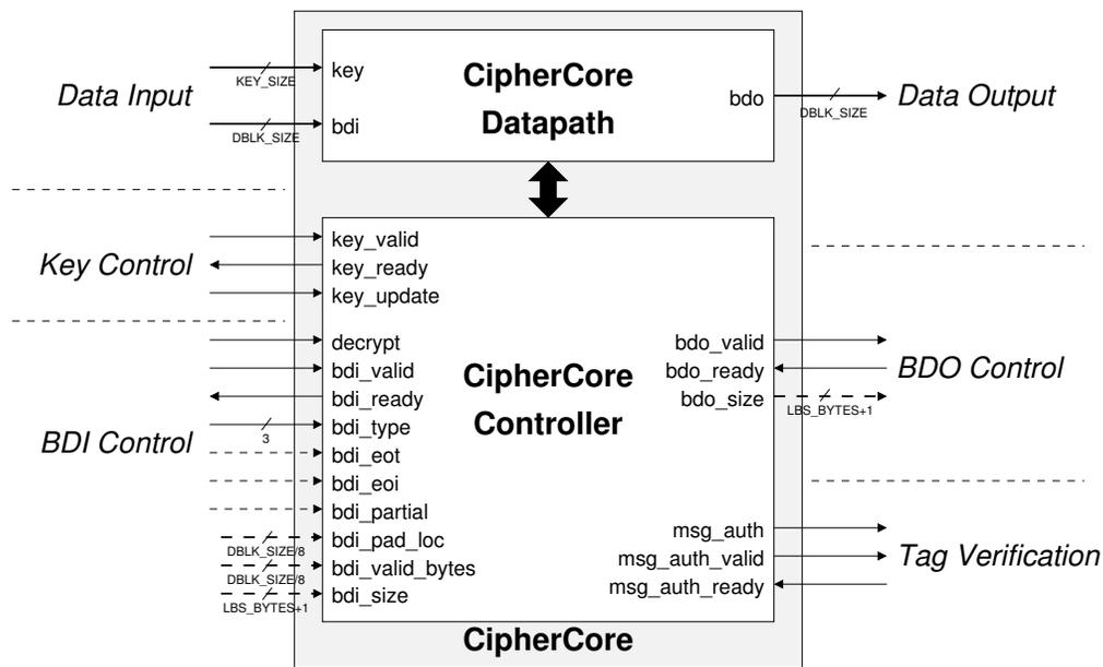
Figure 5.1: Interface of the CipherCore for High-Speed Implementations
