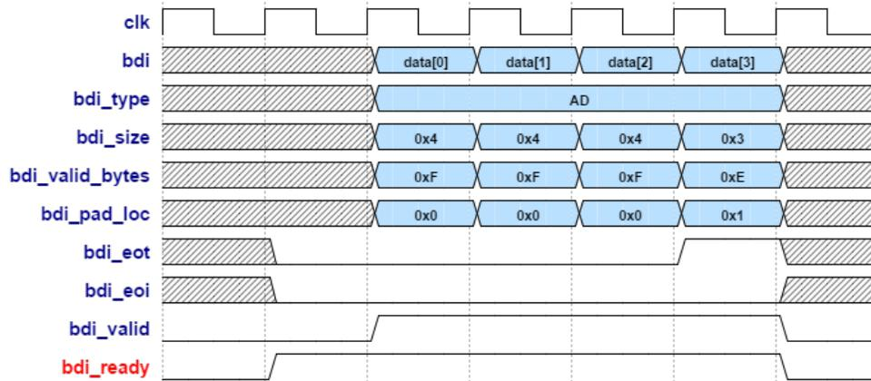
Figure 6.4: Handshake example of loading AD, for  $w=32$ , with data[3] containing the last 3 bytes of AD
