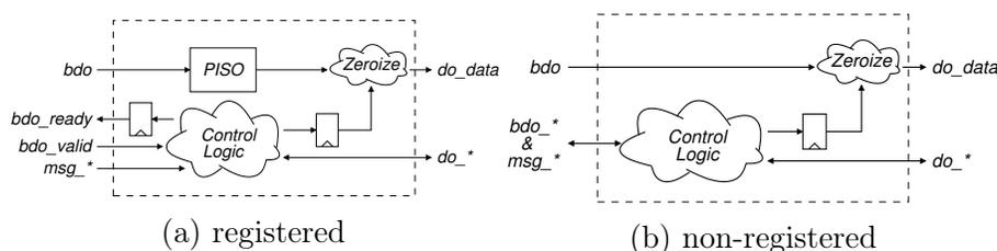
Figure 2.4: The PostProcessor Design. PISO = Parallel-In Serial-Out unit.  $msg_*$ ,  $bdo_*$ , and  $do_*$  stand for all the PostProcessor ports, shown in Fig. 2.1, with the names starting from the respective strings.
