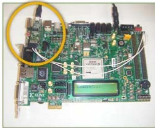
Figure 11: USB Adapter Location on PDIS
