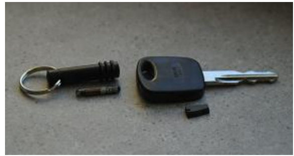
Fig 5.1 At left, an Exxon Mobile Speed Pass both inside and outside its casing. At right, an immobilizer equipped car key. The small chip is embedded into the plastic head of the key.
