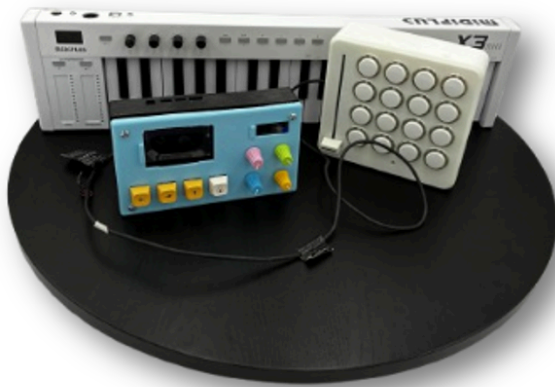
Fig 9. RIFF synthesizer with custom lyric controller and commercial piano keyboard
