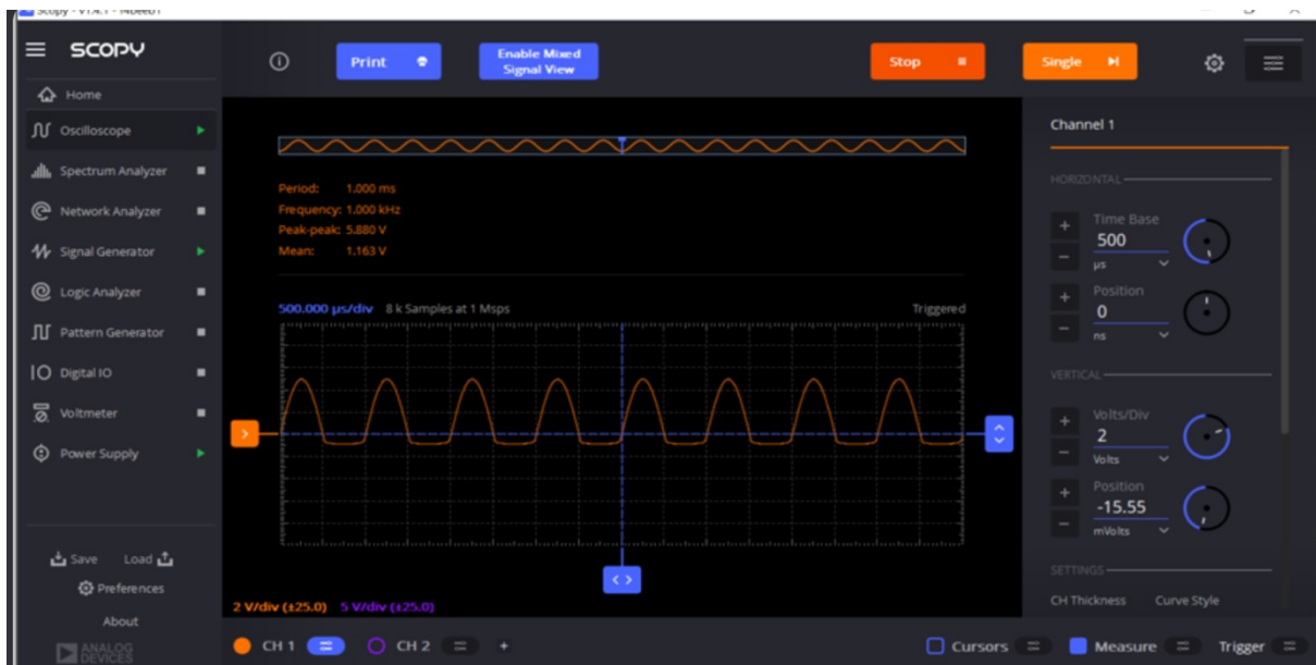
Figure 71: Received output signal through the Bus transceiver
