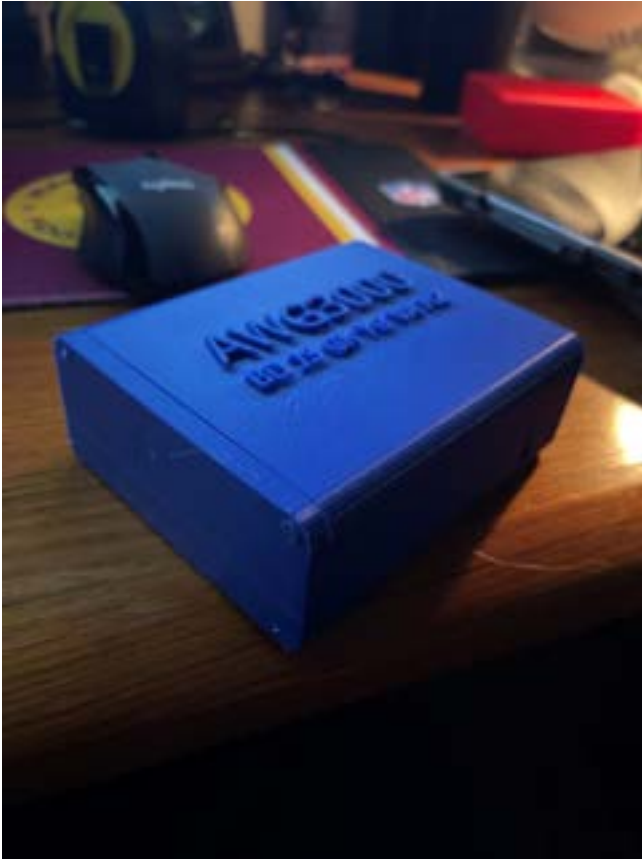
Figure 38: Printed Case Model in PLA - 25% Infill
