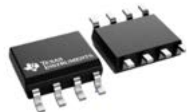
Figure 4 : LMH6506 Variable Gain Amplifier
