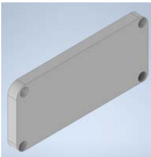
Figure 33: Case Cover - Isometric View
