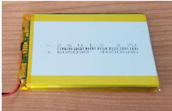
Fig. 22 3.7V 4000mAh Li-ion Rechargeable Battery
