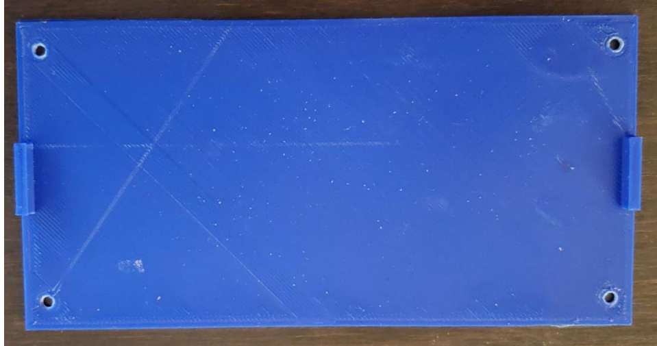
Fig. 46 CAD Design Case Bottom Panel 3D Print 3D Print
