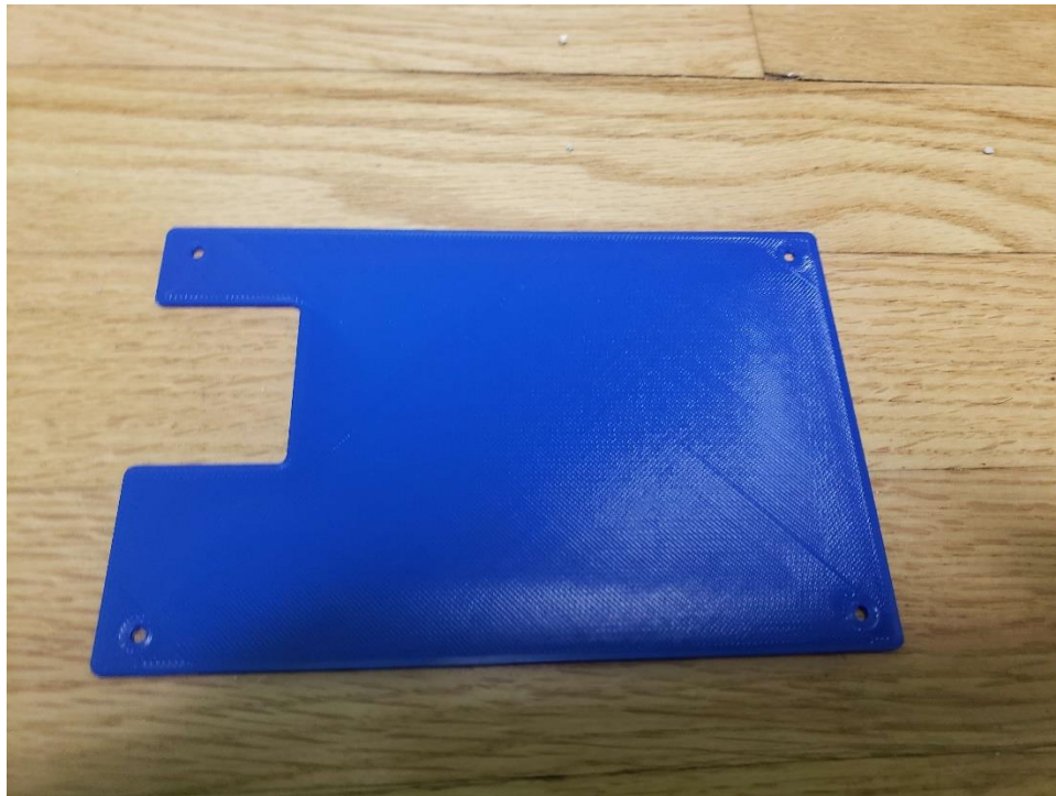
Fig. 47 CAD Design Top Screen Back Panel 3D Print
