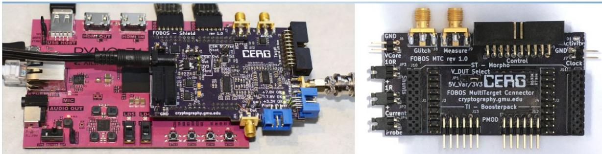
Figure 3.1: PYNQ Board and FOBOS Shield (Left), Multi-Target Connector (Right)
