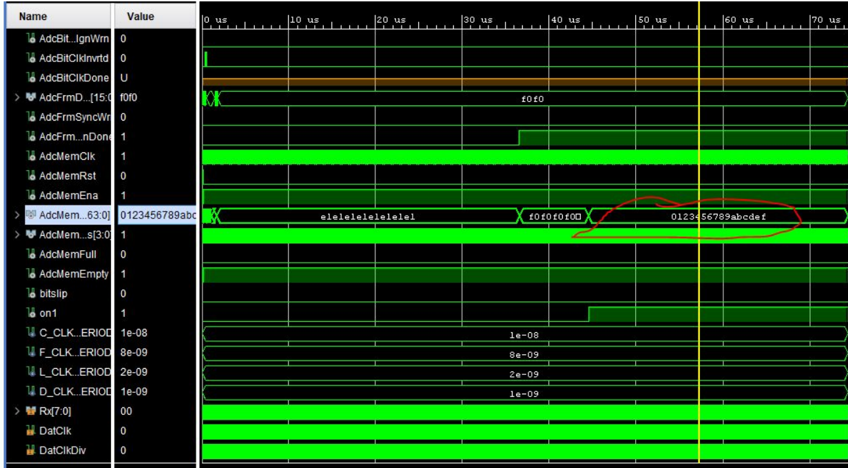
Figure 4.1: Validating deserialization of predictable data in simulation
