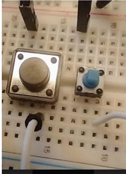
Figure 8: The image above demonstrates a MJTP1234 button (right) which was used in our final prototype.
