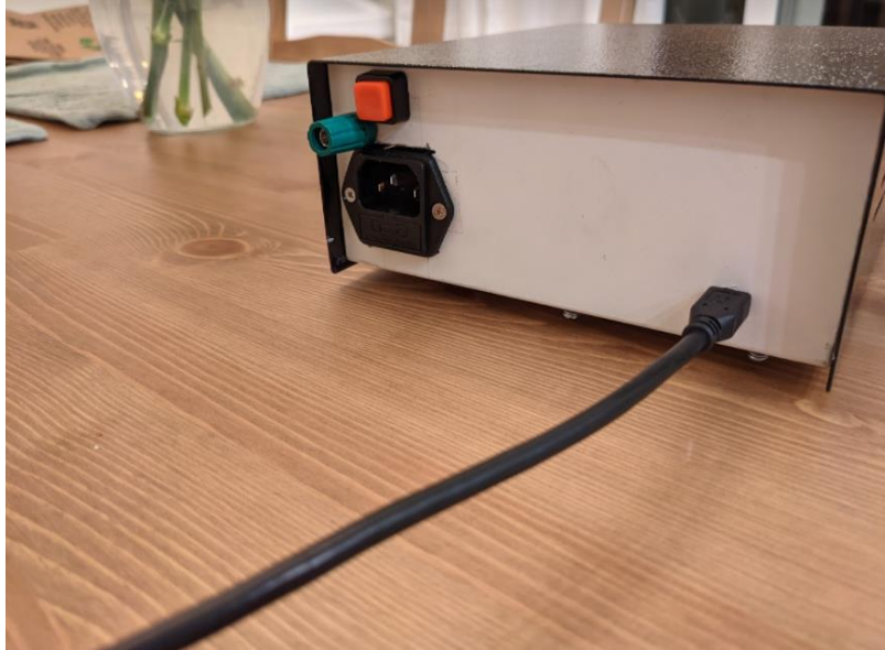
Figure 27: The image above shows the back of the case. The power source is plugged into the back. The orange button is used to turn on and off the case. The green terminal connects to ground, to ground the system.
