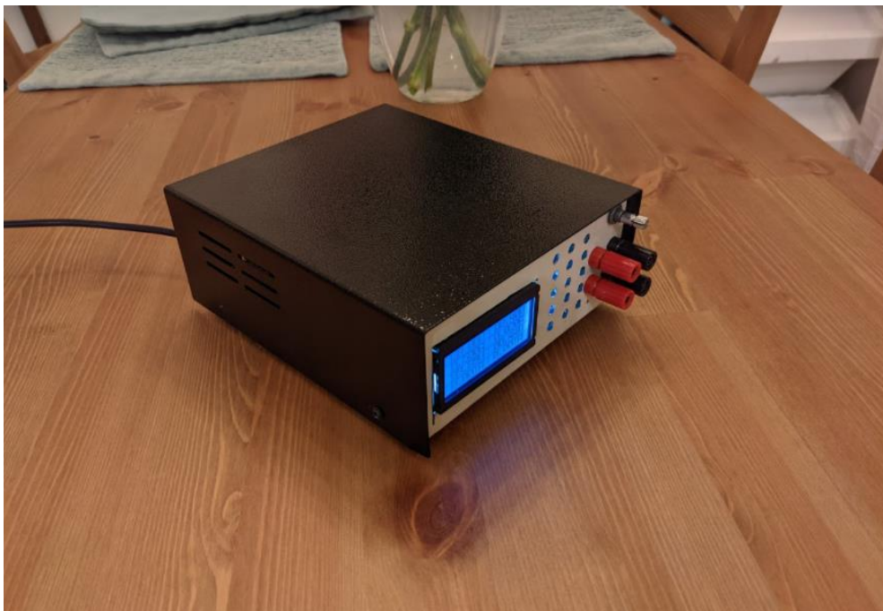
Figure 26: The case above is displayed to show its air ventilation cuts into the side frame.
