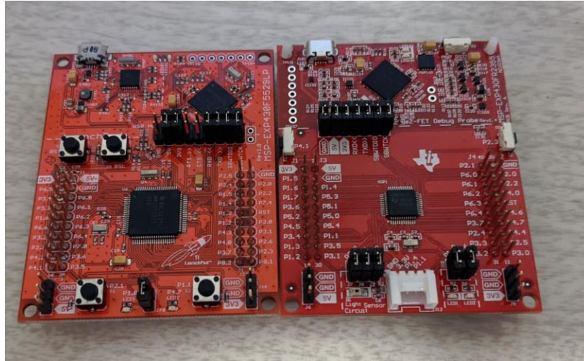
Figure 12: The development boards of both our main MCU and our secondary MCU.
