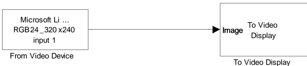
Fig: Schematic for taking input from USB Webcam and displaying on the computer screen.
