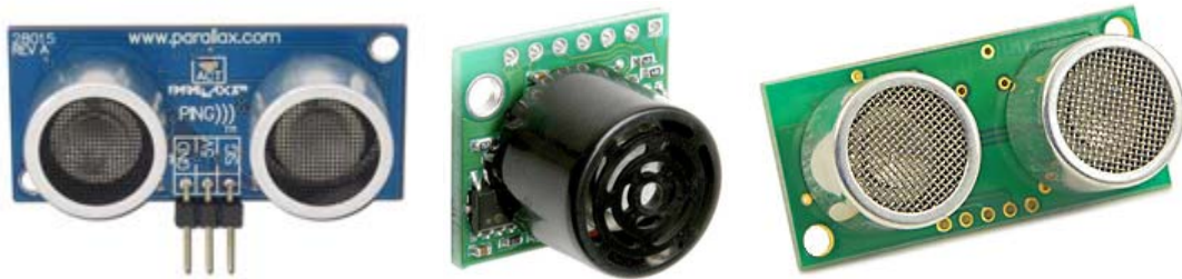
Figure 3: Commercial Off the Shelf (COTS) offerings of ultrasonic sensors at 40 kHz (left to right: Parallax PNG, Maxbotix EZ, Devantech SRF04)
